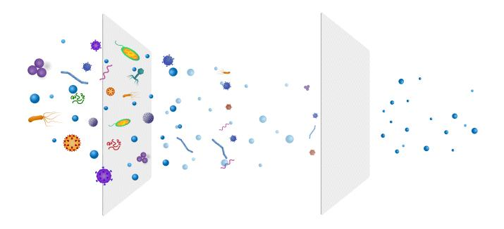
**FILTER STAGE 1** Coarse dust filter G4 of 10 µm **FILTER STAGE 2** HEPA H14 Filter of 0,001µm
